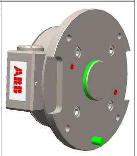
Mount the unit containing the sensor and the adapter flange (or directly mount the sensor when only one adapter is needed) onto the robot side flange using 4 M6x16 class8.8 hexagon socket head cap screws with the 8x20 positioning pin inserted into the corresponding positioning hole in the robot side adapter flange.
